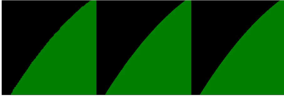
Figure 12. Quality versus texture read count. Left: One Texture Read (one bilinear sample). Middle: Two Texture Reads (two linear samples). Right: Three Texture Reads (three nearest neighbor samples).
